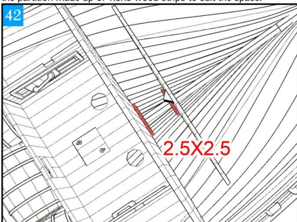
Figure 42. The beams for the ammunition magazine is made up from 2.5x2.5 wood strip as shown
