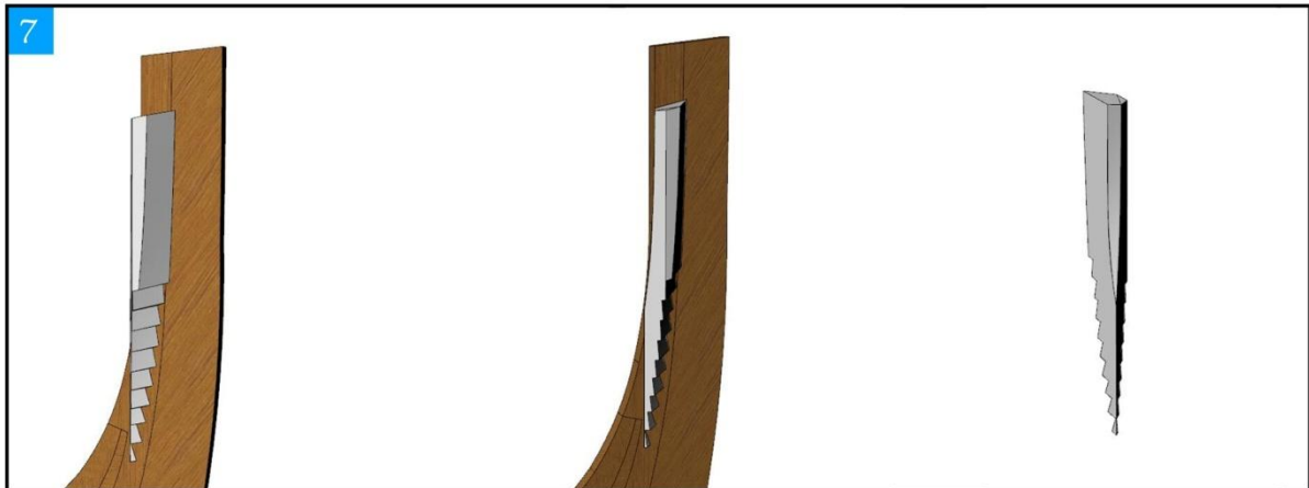
Figure 7. We next move to the bow or “cant” frames that go together to form the round bow. To help you visualize the shape of cant frames and how they fit to the stempost, the illustration shows three different views of . No.1 bow frame. Note how complex the shape is a tapered wedge that tapers in two faces, with notches cut for planking. When the cant frames are stacked together they form a curved face.
