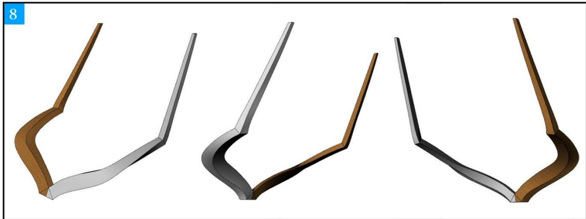
Figure 8. shows the stern side counter timbers, which are processed by CNC. Three angles are selected for observation. The stern timbers are built according to the plans and once again, careful checking and rechecking of their shape and angles is vitally important.
