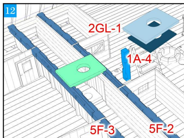
Install the beam, adjust and install the winch base
